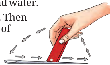
Fig. 4.7(a): Making an iron needle a magnet
